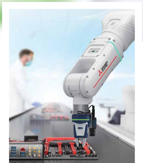
The MELFA Assista is suitable for handling small loads of up to 5 kg.
