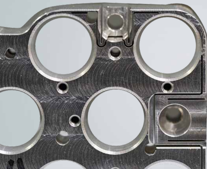
Erosion contour for the flexible alignment of the plate plane
