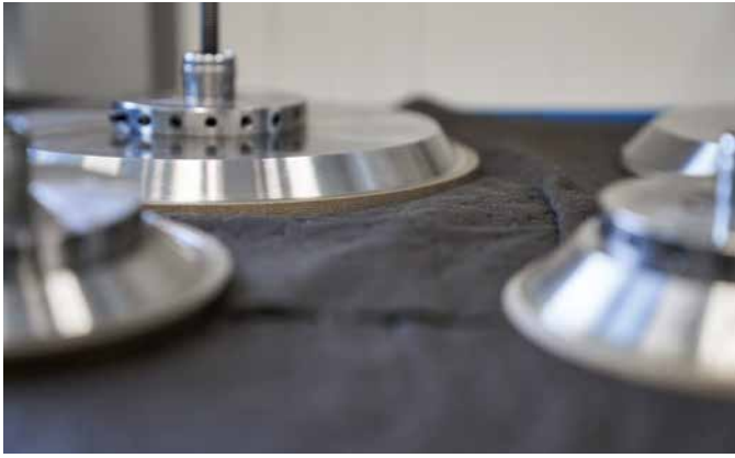
Diamond grinding wheels before the eroding process
