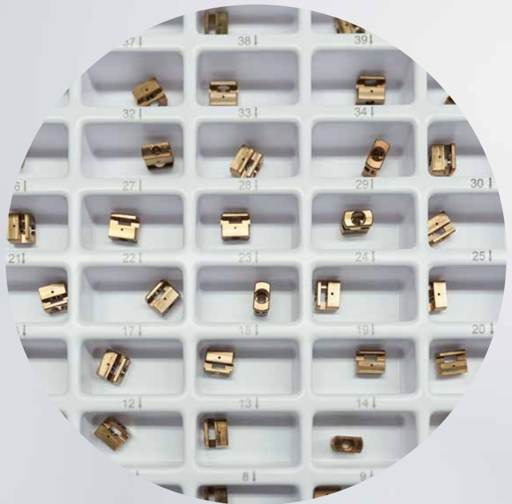
Blanks with labelled packaging for the assignment of serial numbers
