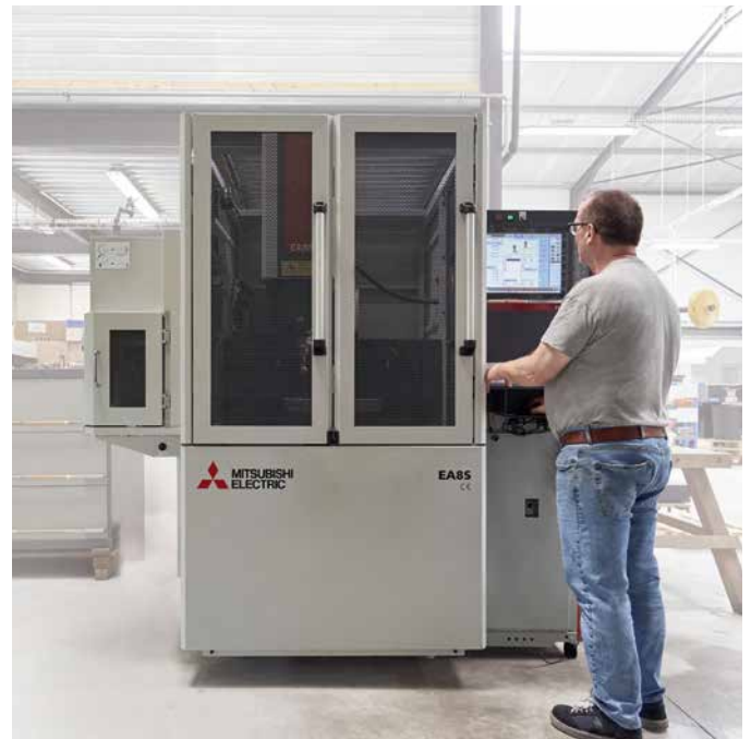
The Mitsubishi Electric EA8S die-sinking EDM system that went into operation at the same time as the MV1200R
