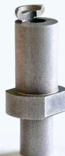
Winding mandrel for lamp filaments
