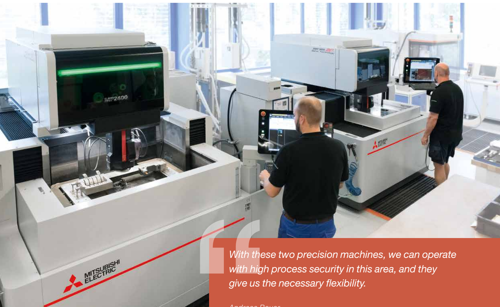
The two Mitsubishi Electric machines in the EDM section of the toolshop
