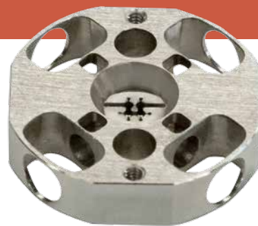
Body of an HF assembly – produced on the MP1200 from Mitsubishi Electric
