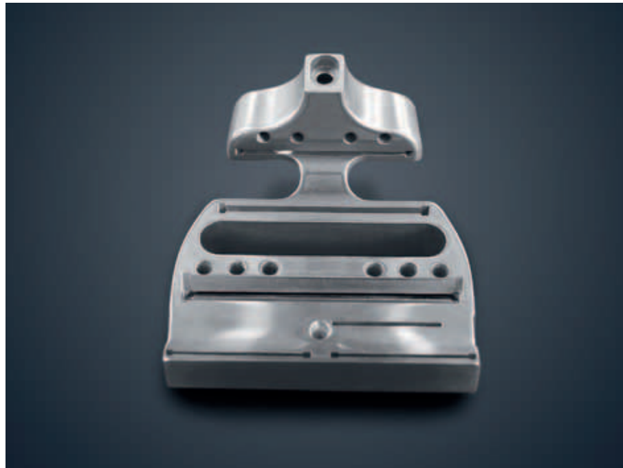
Cutting guide from the medical technology field with incisions at certain angles that SPEMA has wire-cut with the aid of a B-axis.
