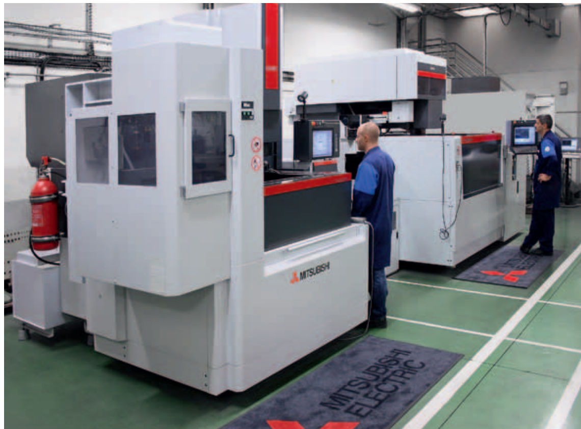
Sogameca produces most parts by getting the desired workpiece into shape initially with die sinking and then cutting the material with wire EDM.
