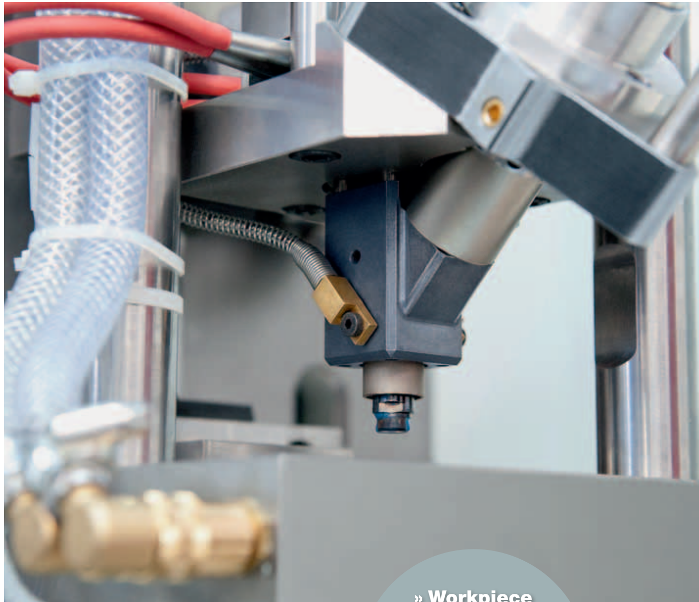
Installed in the micro-injection moulding machine, a machine nozzle is mounted on the thread of the two-stage injection cylinder.
