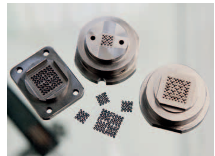
The plastics parts produced in the micro-injection moulding machine weigh only a few milligrams, yet their complexity is exceptionally high.
