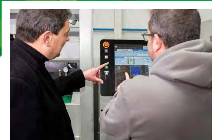
On the Natural User Interface (NUI), the touchscreen is similar to that of a tablet PC, which greatly simplifies navigation through the various functions.
