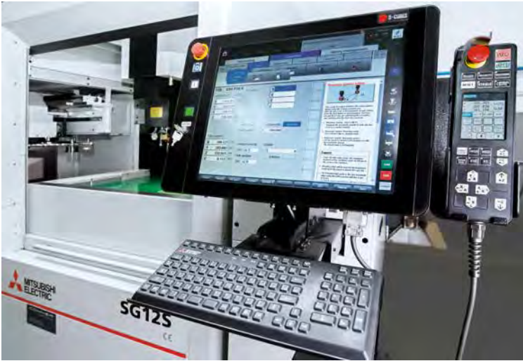
With step-by-step guidance, less experienced users can navigate their way through complete process control. In addition, the intuitive hand control makes it easy to adjust the part in the machine.
