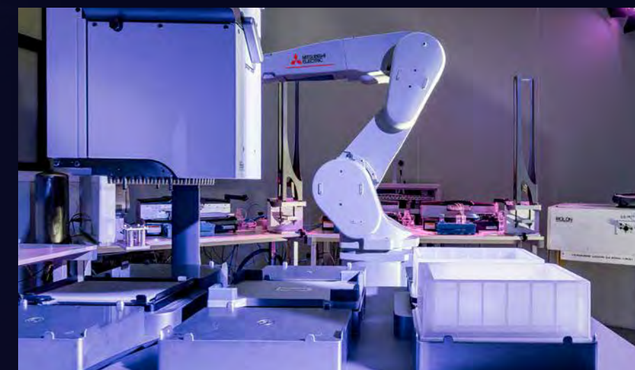
The Mitsubishi Electric robot is the central component of the system. It continuously operates the analytical equipment on the basis of specifications, conducting 15,000 tests per day, 7 days per week.
