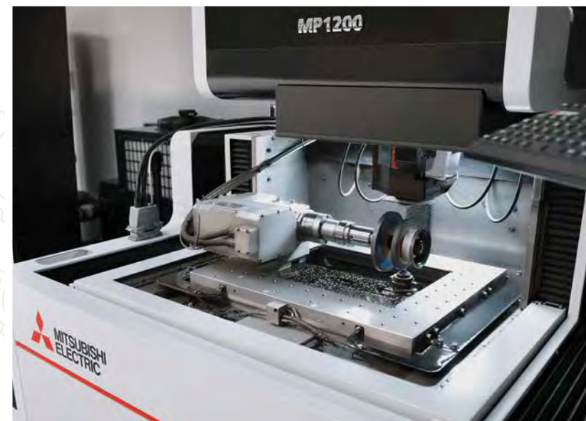
Enhancing precision and effectiveness while cutting costs can be achieved with metal-bonded grinding wheels machined on Mitsubishi Electric EDM-DRESS.
