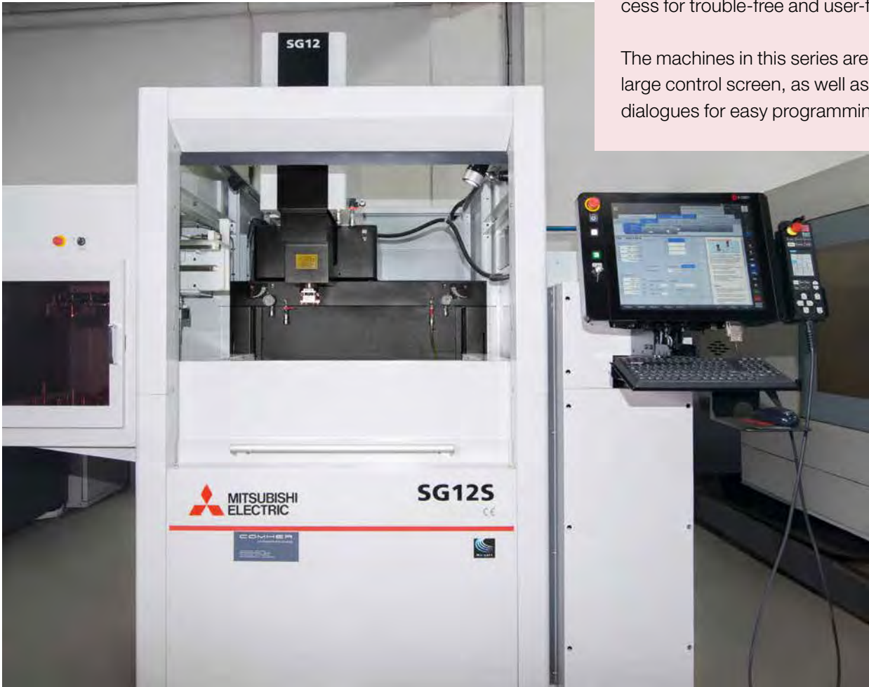
SG12S Mitsubishi Electric die-sinking EDM machine. Compact and user-friendly design.
