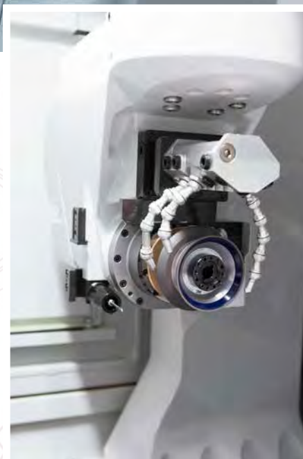
Grinding tool EDM-dressed ready for production
