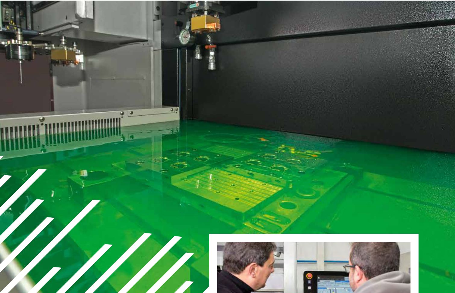
Good accessibility and user-friendliness thanks to the three-sided, low-erable work tank – for easy handling.
