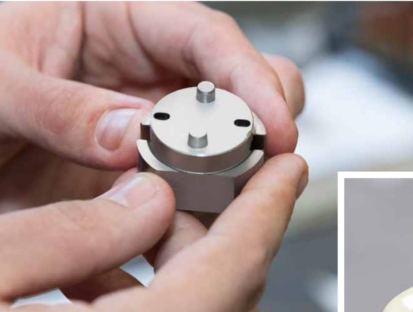
Fixture for wire-cutting mould inserts. HT Tooling can also respond quickly to customer requests when it comes to very small series.
