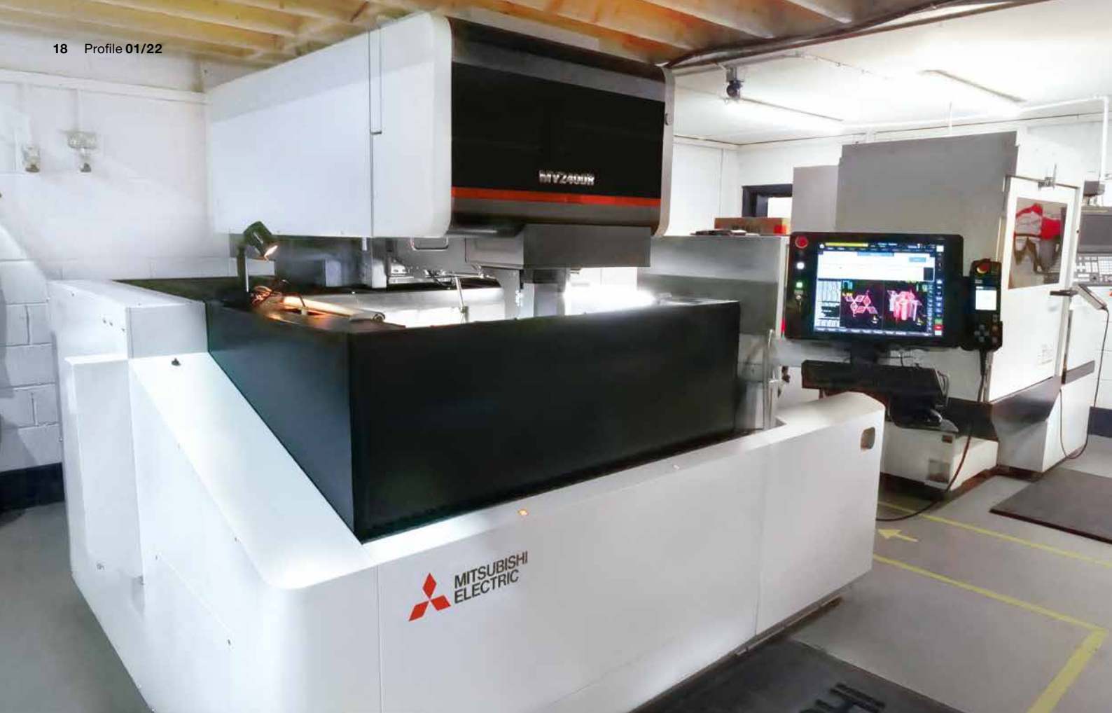
The machines have glass linear scales right next to the workspace. This enables maximum accuracy.
