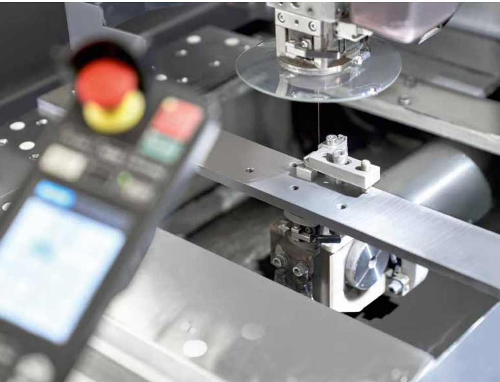
A clamped specimen in the installation space of the MV1200S shortly before the start of the process
