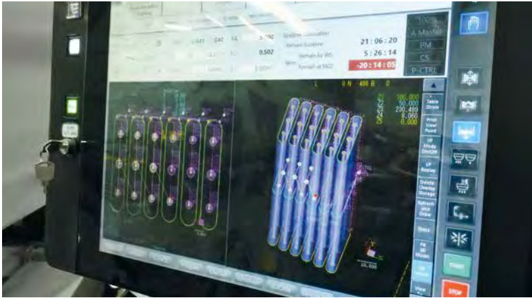
The new user interface with a 19-inch touchscreen offers integrated CAD/CAM programming to optimise the work process.
