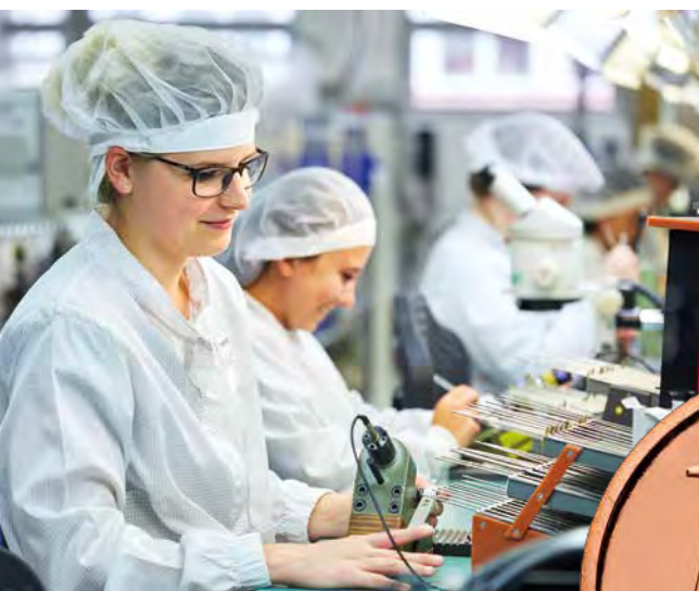
The precision roller bearings are tested and assembled in the cleanroom.
