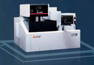
MV2400R Connect Machine height 2150 mm Surface finish in the standard version Ra 0.25 µm MV2400R Z+ Connect available: Machine height 2380 mm Travel X: 600 mm, Y: 400 mm, Z: 425 mm Max. workpiece dims. (WxDxH) 1050 x 820 x 420 mm Maisart Report on page 86
