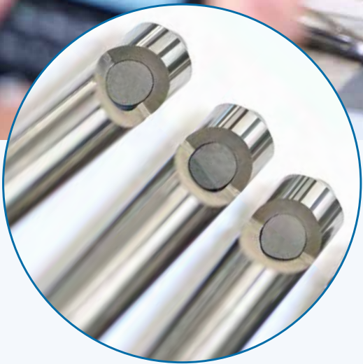
The plugs at the end of these tungsten carbide nozzle tubes cause the impinging sand particles to be deflected sideways in order to clean narrow interior cavities.
