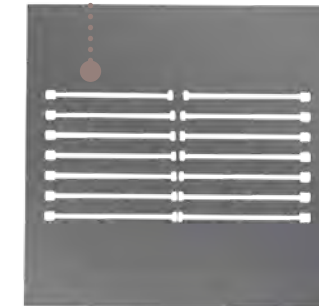
0.4 mm template made of 1.4301 with web widths decreasing from 1.0 mm to 0.03 mm
