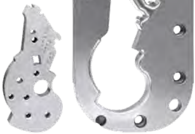
The punch and die for a sheet metal part are cut by wire erosion from hardened tool steel several centimetres thick.
