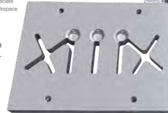
Minimalistic: To produce prototypes or small pilot series, the simplest punching and forming tools are often sufficient.
