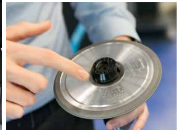
Profiled grinding wheel with DataMatrix code
