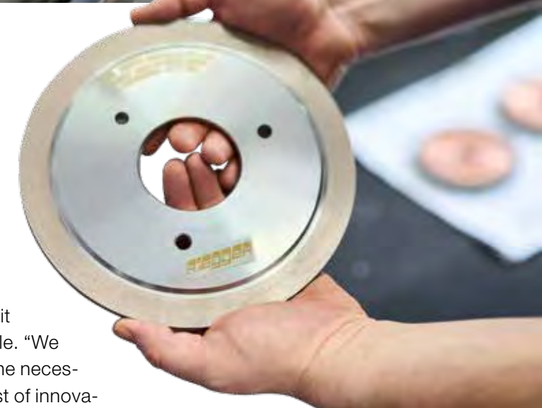
The specialists at Riegger individually profile standard grinding wheels with diamond or CBN as a solid basis.
