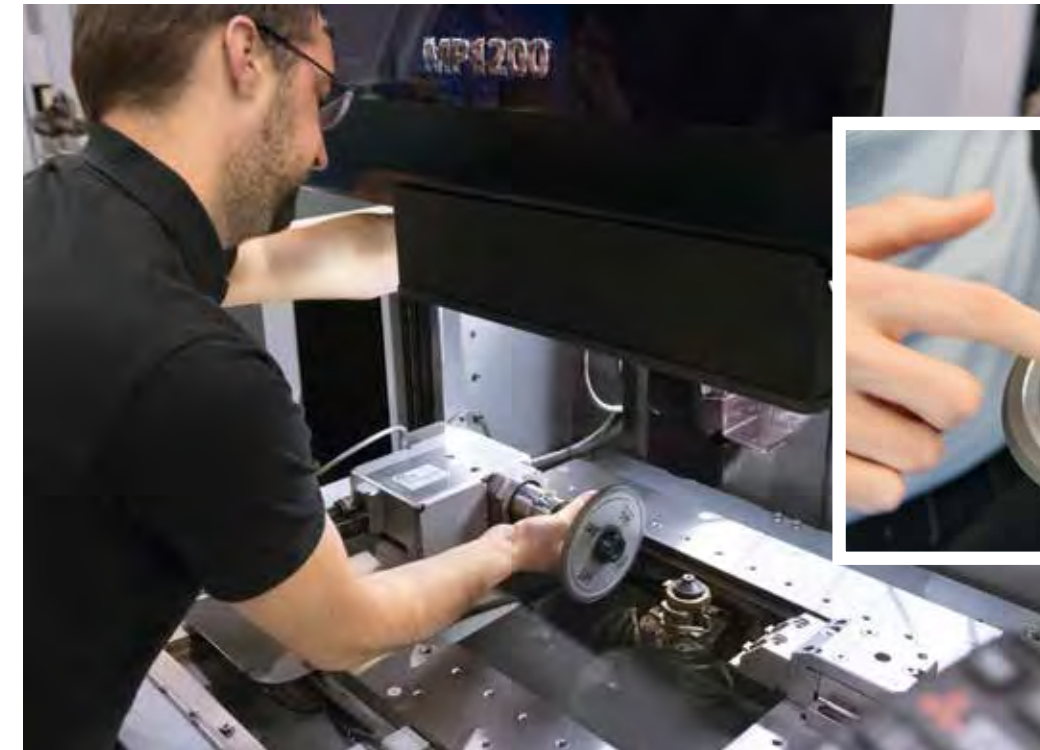
Clamping the grinding wheel in the ITS spindle in the MP1200 Connect's spacious workspace
