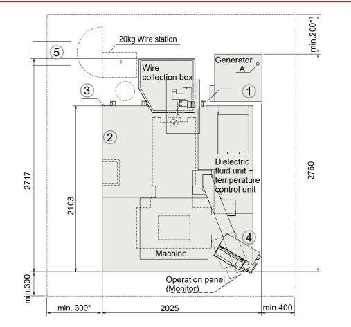
\* is min. 700, when the 20 kg wire spool unit is mounted
